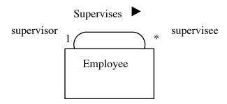
Note: Care must be used in drawing a diagram to distinguish between the name of an association and role names. The latter should be drawn near the end of the association line; the former far enough from the ends to be clear that it is not a role.
