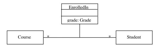
(Note the use of the three sets of lines in the box representing the association class, to make it crystal clear that this is a class.)
